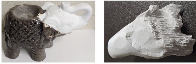
**Figure 13:** The 3D print of the elephant head does not make a perfect join with the elephant (left) due to uncertainties introduced by the nozzle diameter, and the presence of support structure remnants on the fracture surface (right).
